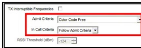
The screenshot shows the 'TX Interruptible Frequencies' settings. A red box highlights the 'Admit Criteria' and 'In Call Criteria' dropdown menus. 'Admit Criteria' is set to 'Color Code Free' and 'In Call Criteria' is set to 'Follow Admit Criteria'. Below these, the 'RSSI Threshold (dBm)' is set to -124.
